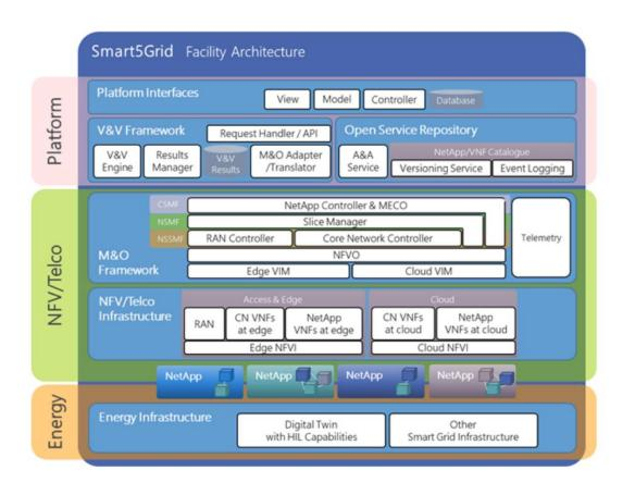
Smart5Grid's functional Architecture consists of discrete layers:
