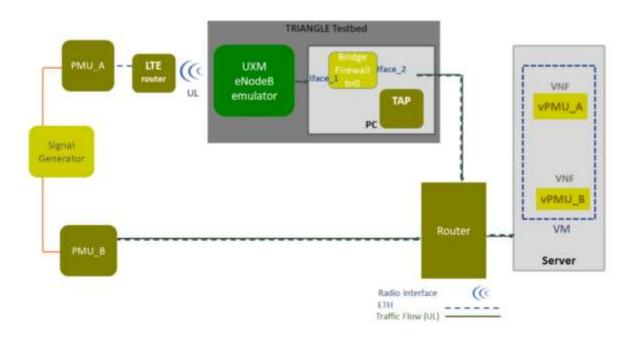
TRIANGLE testbed is an End-2-End (E2E) testbed which allows flexibility and reconfiguration for realistic testing scenarios:
